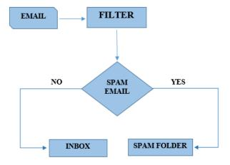
Fig2. Flow chart of Spam filters
